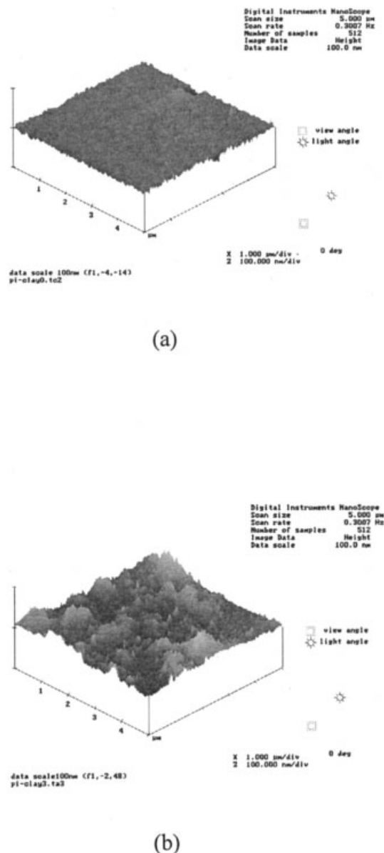
Figure 5 Atomic force microscopy (AFM) studies of (a) PI and (b) CLPI3.
